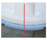
For technical reasons, do not place a hole in the center of the bow bend or in the center of the stern corners.
